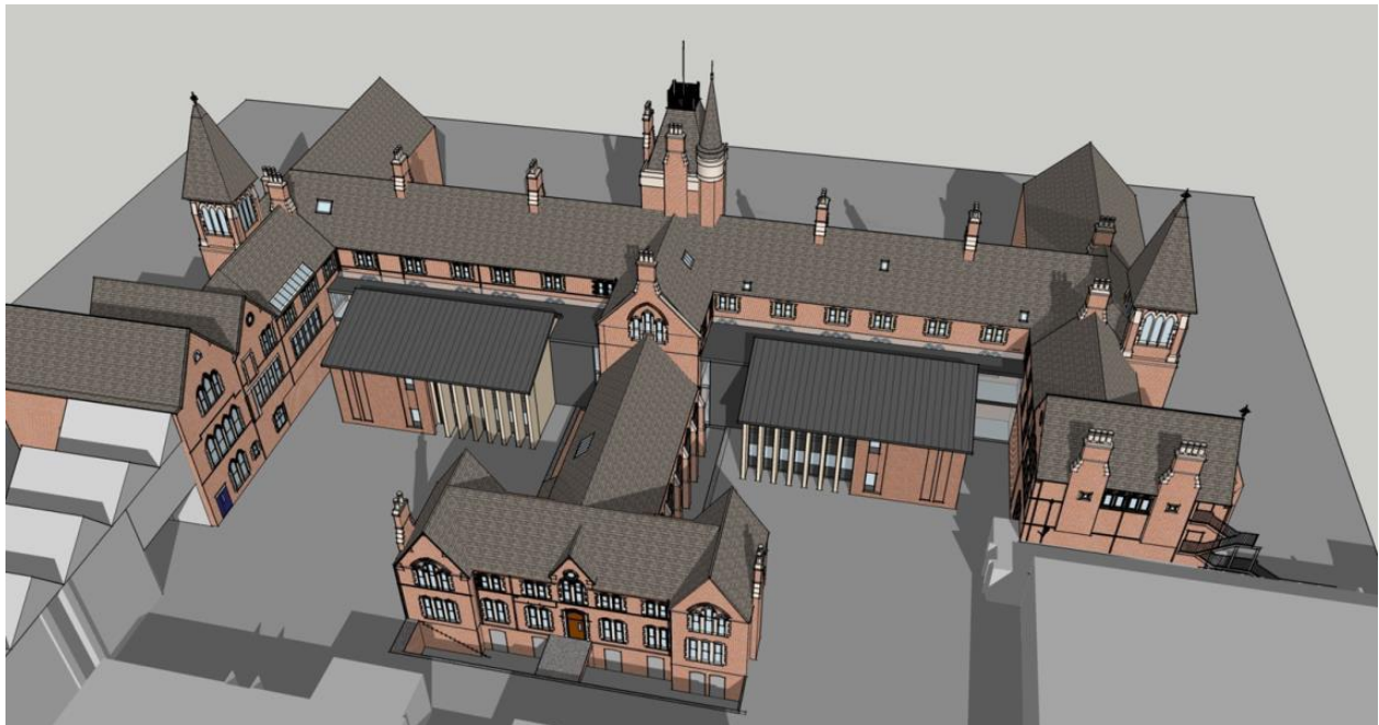
Rear elevation showing new classroom extension
